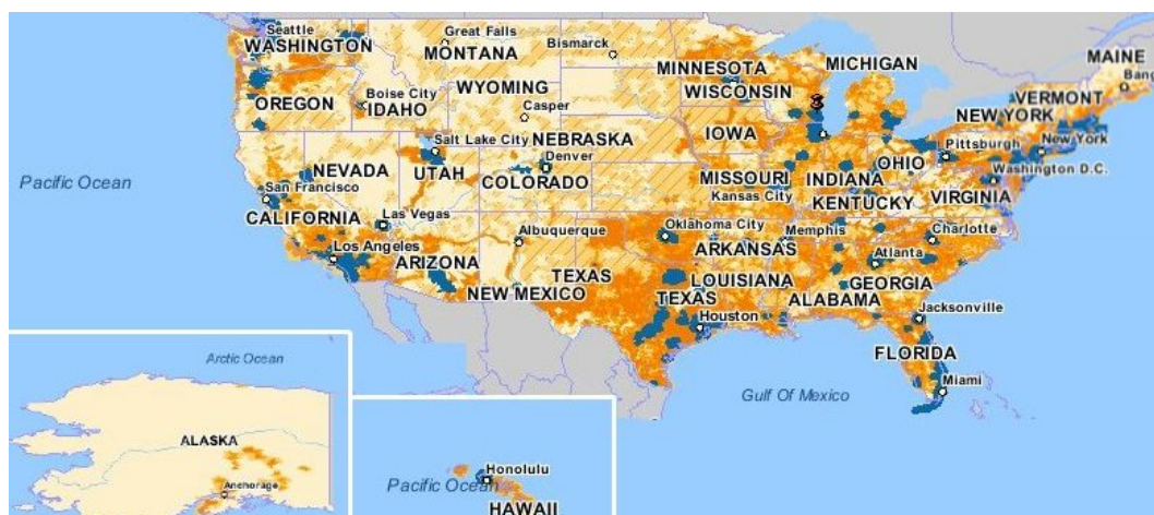
Figure 1.3: AT&T's coverage of the United States, July 2008. Blue is 3G; dark and light orange are EDGE and GPRS; and banded orange is partner GPRS. The rest is 2G or no coverage.
