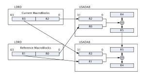
Fig. 3. SAD calculation using the USADA8 instruction.
