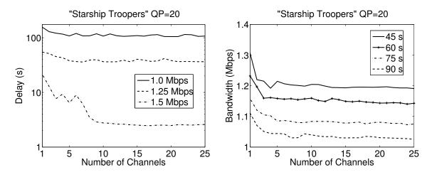
Figure 3: Delay at varying bandwidths and bandwidth at varying delays for "Starship Troopers"
